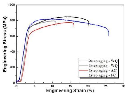
**Fig.1** Tensile curves of Haynes 282 at 750°C for the various heat treatment
