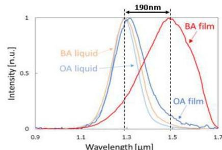
**Fig.2** PL spectra of BA-treated and OA-treated PbS QD in liquid and film, respectively.
