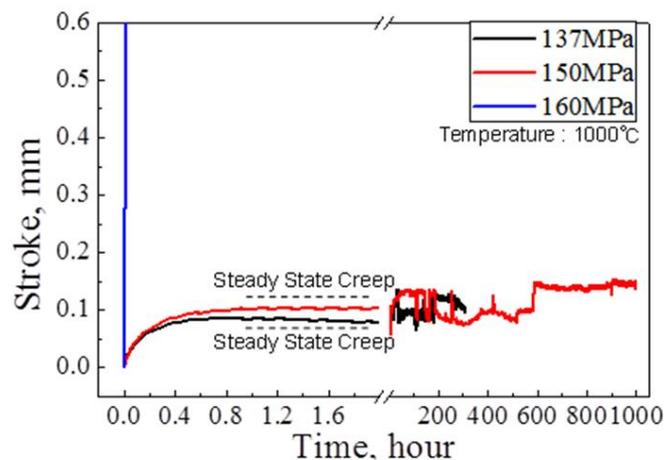
Fig.1 Creep curves of the fiber-reinforced self-healing ceramics at 1000°C
