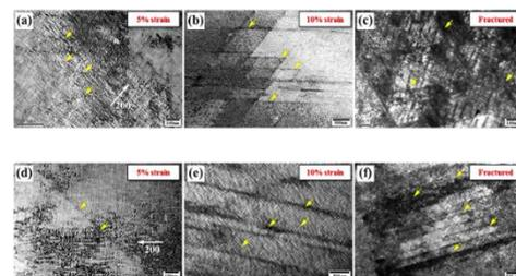
**Fig.2** Evolution of deformation microstructure of Si free and 1% Si added steel by TEM.
