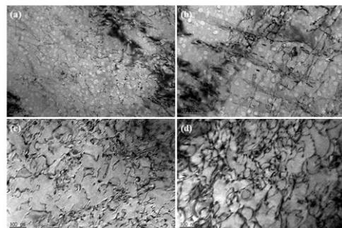
**Fig.2** TEM Bright field images showing the dislocation behavior after tensile test at 750°C : (a) 2step aging heat treatment following water cooling, 1step aging heat treatment following (b) water cooling, (c) air cooling and (d) furnace cooling.
