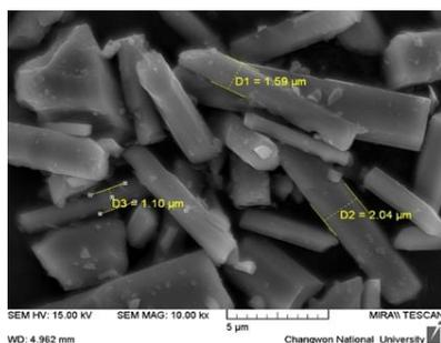
**Fig. 1.** FE-SEM image of potassium titanate whisker synthesized by Flux method at condition 5 with flux X & quenching O
