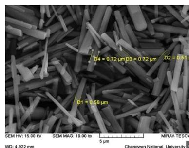
**Fig. 2.** FE-SEM image of potassium titanate whisker synthesized by Flux method at condition 5 with flux O & quenching O
