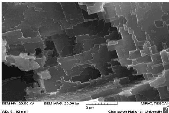
**Fig.1** FE-SEM image of Al 3003 with HCl(25%) at 30°C for 7min
