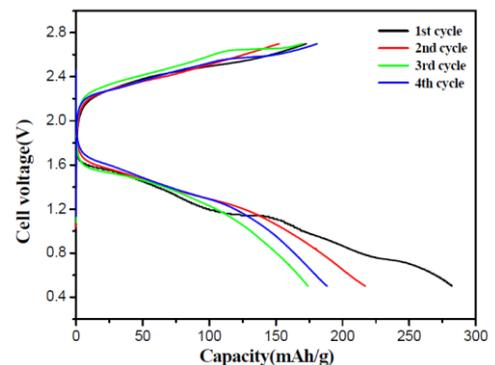
**Fig.2** Galvanostatic charge/discharge voltage curves of Case 2
