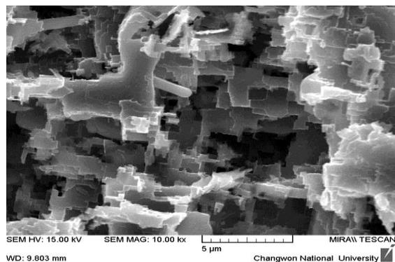
**Fig.2** FE-SEM image of Al 3003 with HCl+FeCl<sub>3</sub>(33%) solution at 30°C for 7min
