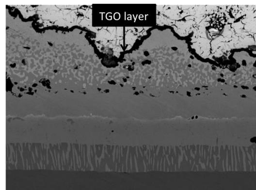
**Fig.2** Scanning electron micrograph of the TBCs heat exposed at 1273 K for 100 h.
