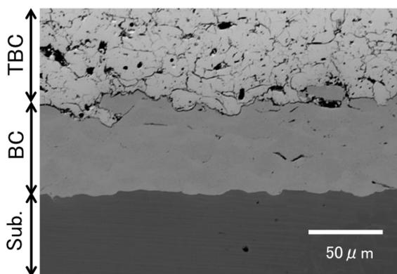
**Fig.1** Scanning electron micrograph of as-deposited TBCs.
