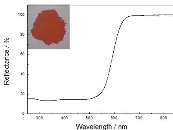
**Fig 2.** UV-vis diffuse reflectance spectrum of  $K_3V_5O_{14}$  pigment after annealing treatment at 400°C.
