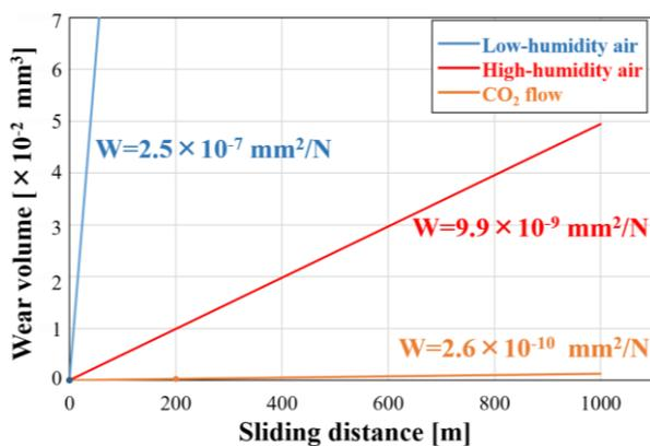
Fig.1 Wear volume of AlN ceramics under different atmosphere and specific wear rate
