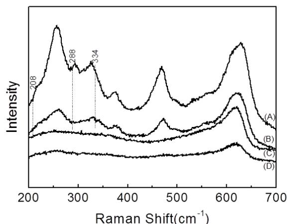
**Fig.2** Raman spectra (A) anode(Ni-YSZ cermet) after exposure to H<sub>2</sub> containing 25ppm H<sub>2</sub>S, (B) anode(Ni-YSZ cermet) after exposure to H<sub>2</sub> containing 10ppm H<sub>2</sub>S, (C) YSZ pellet, and (D) anode(Ni-YSZ cermet)
