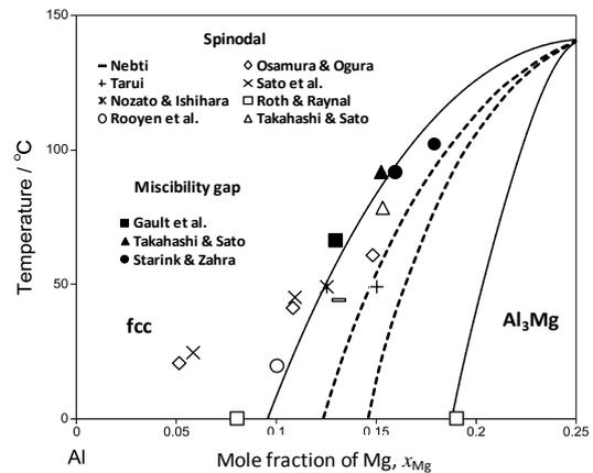
**Fig.2** Calculated miscibility gap (solid lines) and spinodal lines (broken lines) of GP zones (Al<sub>3</sub>Mg). Experimentally reported data is also shown by symbols.
