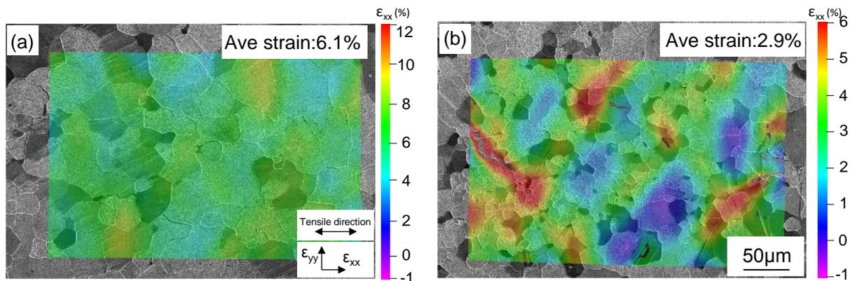
Fig.1 Strain distribution along tensile direction in tensile deformed specimen at 293 K (a) and 77 K (b).
