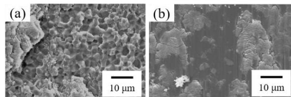
Fig.2 SEM images of worn surfaces of AlN ceramics after ball-on-disk test in (a) low humidity air and (b) high humidity air.
