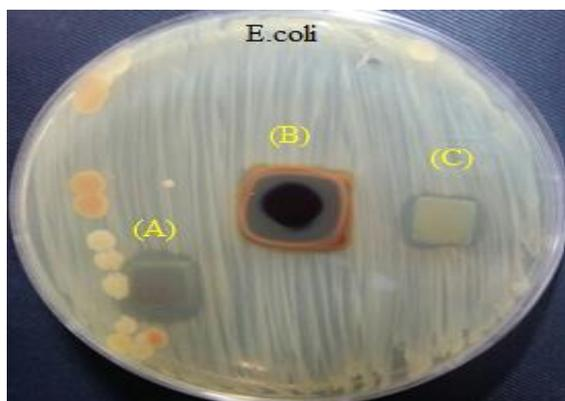
**Fig.1** Disk diffusion test of synthesized by Ag-SiO<sub>2</sub> nanoparticles and inorganic binder; (A)5g, (B)0g and (C)2g
