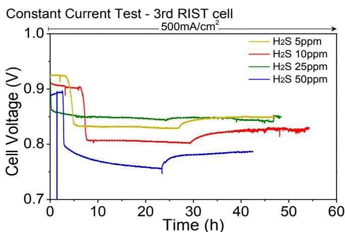
**Fig.1** Constant current test with hydrogen sulfide contained fuel respectively 5ppm, 10ppm, 25ppm, and 50ppm at 500mA/cm<sup>2</sup>
