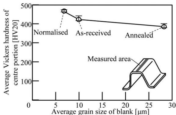
**Fig.1** Effect of grain size of steel sheet before hot stamping on Vickers hardness after die quenching in hot stamping using resistance heating for  $\nu = 275$  °C/s and  $t = 0$  s.
