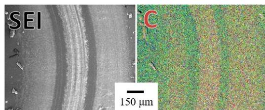
Fig.3 SEM image and EDS image of worn surface of AlN
