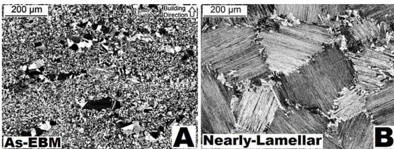
Fig.1: Microstructure of Ti-45Al-2Cr-8Nb A: as-EBM and B: Nearly-Lamellar after heat treatment
