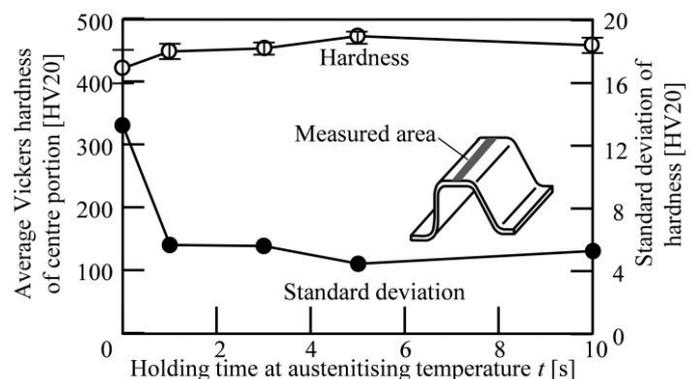
**Fig.2** Effect of holding at austenitising temperature on Vickers hardness and standard deviation for  $\nu = 275$  °C/s.
